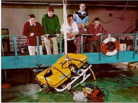
Systems students working with an underwater exploration vehicle: the aim of the project is to enable the vehicle to operate autonomously, eliminating the need for the umbilical cable linking it to an operator at base. The technology being developed here is equally applicable to Unmanned Air Vehicles and the next generation of combat aircraft.
