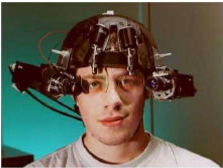
This project involved Systems Students developing a headset and supporting equipment that could be used by disabled people to control a PC by eye movement alone. This project drew on many fields of study, including computing, electronics and virtual reality. If developed further, this could be a useful technology for use in a future fighter aircraft cockpit, easing the pilots workload in a difficult and busy environment.
